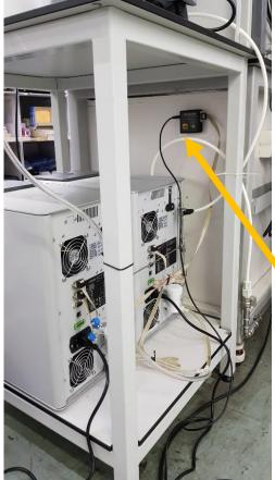
Water system to allow easy top up of the 5L Tank
