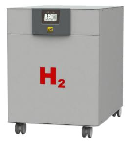
Hydrogen generator that can generate high-purity hydrogen gas at flow rates of 4 L/min, 8 L/min, 16 L/min, and 20 L/min. The HG PRO M includes a new long life multilayer electrolytic cell with polymeric membrane (PEM) using ultra pure water. No acid or alkaline solutions are used.
