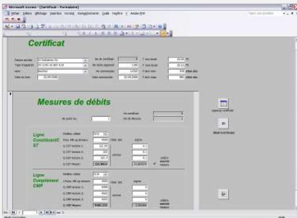
For each series of measurement, a certificate of calibration includes : the customer ID, the measured device, operator, the employed method, Fluidics, uncertainty of measurement, conditions of measurement and results of measurements is automatically generated, thus making it possible for customers to ensure total traceability of their Flow and concentrations measurements
